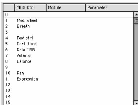
The screenshot shows a window with three columns: MIDI Ctrl, Module, and Parameter. The MIDI Ctrl column contains numbers from 0 to 15. The Module column is empty. The Parameter column contains the following text: Mod. wheel, Breath, Foot ctrl, Port. time, Data MSB, Volume, Balance, Pan, and Expression. The list is scrollable, with a vertical scrollbar on the right side.
