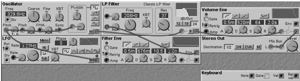
Notice that there are two ways to cable one output to two different inputs: in parallel (two cables from the output) or in series (one cable from the output to the first input and another from the first input to the second input). Since the connections are functionally the same, choose the most convenient one when creating your own patches.
