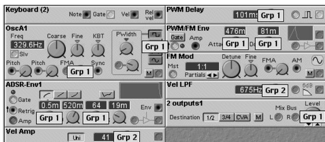
The affected parameters are all labeled ›Grp 1‹ in the illustration. In the editor, they are also red. You can ›morph‹ these controls on-screen by moving the red morph knob with the mouse and/or you can assign a MIDI controller or Modular front-panel knob to the morph. (We've assigned both knob 1 and the mod wheel to it.)
