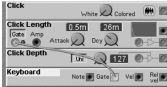
In all humility, here's a perfect example that—in the Modular—imagination can prevail over a perceived limitation: the click signal doesn't roll right onto the audio rails—we route it to the FM input of all sine generators because with this configuration, the sine tones start up with a very distinctive clicking sound—which is a vast improvement over using the noise signal directly.
