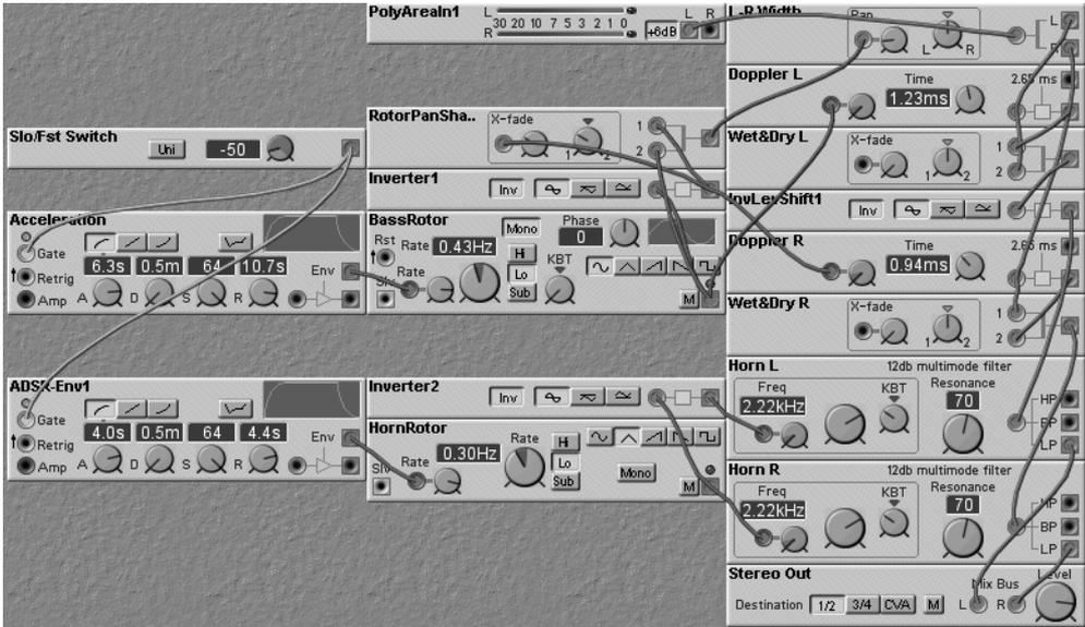
This part of the setup is truly hardcore. The Leslie sound is derived from the composite signal of a bunch of modules that were painstakingly micro-tuned so that—when added up—deliver a decent Leslie sound. Accurate electronic Leslie simulation is generally regarded as a higher form of art, so you can imagine what it takes to squeeze something convincing out of a purely modular synthesizer.
