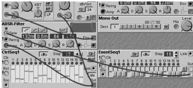
Only the purple cables should be visible. You can see that the output of CtrlSeq1 is cabled both to the amp input of the ADSR-Filter envelope and to the res input of the filter. The envelope output is cabled to the frequency mod input of the filter. The control values coming from this sequencer will therefore control the amount of the envelope applied to the filter frequency and the filter resonance. Notice also that the
