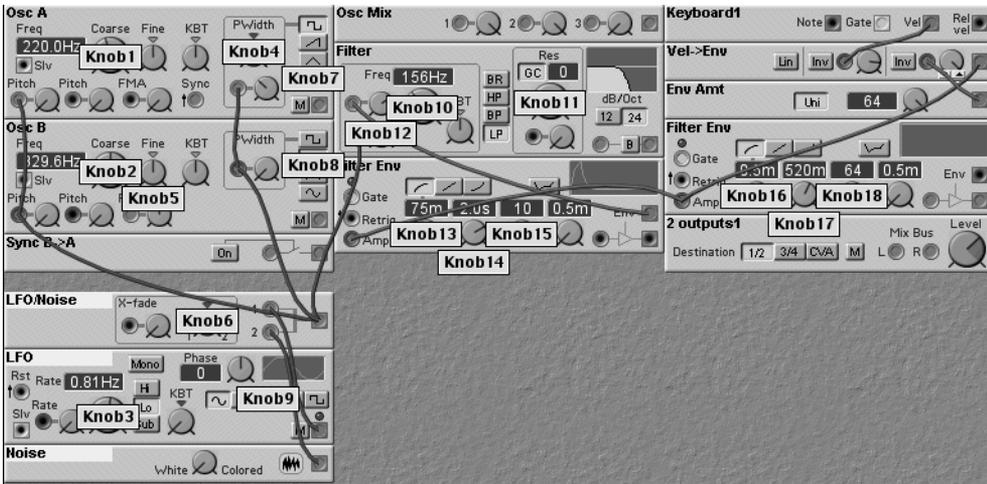
This is a basic two oscillator synth with a multi-mode filter, plus LFO/noise modulator and two ADSR envelopes. It is reminiscent of the early portable synths like the Minimoog, Arp Odyssey and Oberheim Xpander. The concept is taken to its 21st century extreme in the next model, but you can do a lot with just this basic mini-model. For starters, just twiddle the knobs then adjust the on-screen controls to add modulation and finally begin adding new modules as the spirit moves you.
