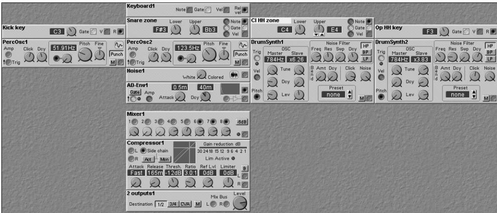
In this patch, you can see that four components of a drumkit are arranged side by side: kick, snare, closed hihat and open hihat, playable by the keys C3, F#3 to A#3, C4 to E4 and F3, respectively. On the Modular keyboard, you'll find these keys
